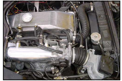
1975 FI System (seen retrofitted in Opel GT)
