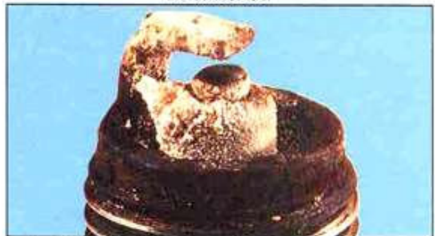
Ash deposits – Light brown deposits encrusted on the electrodes and insulator, leading to misfire and hesitation. Caused by excessive amounts of oil in the combustion chamber or poor quality fuel/oil
