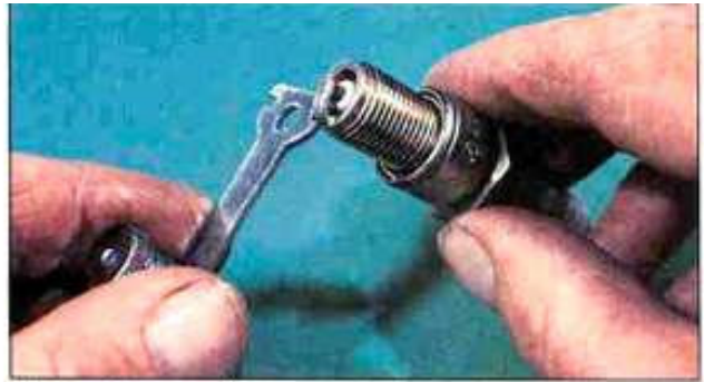
Electrode gap adjustment – bend the side electrode using the correct tool
